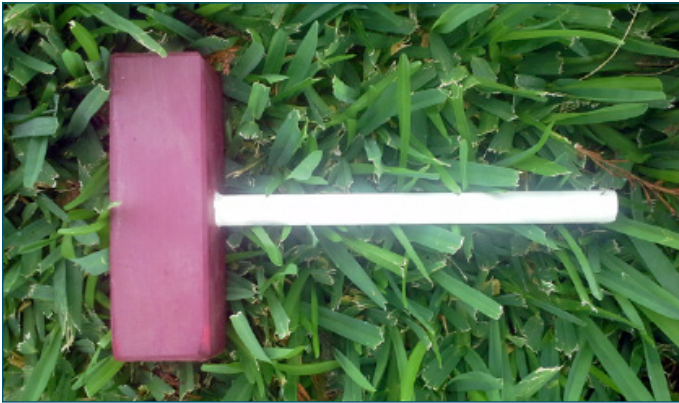
Figure 6. Dowel rod and handle used as a tool to test for soil hardness. Photo credit: Bill Ree
