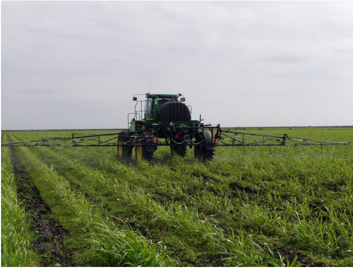
Figure 7B. (B) boom sprayer Credits: UF/IFAS Pesticide Information Office
