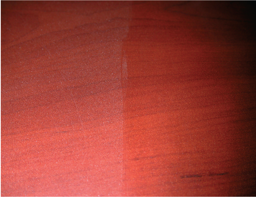
Figure 12. Dusts should be applied so that a very thin film is visible on the treated surface (left side).
