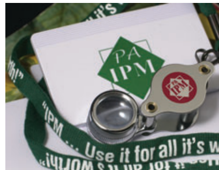
Figure 2. A hand lens is a critical IPM tool for proper pest identification. Choose a hand lens with 10x power or greater.
