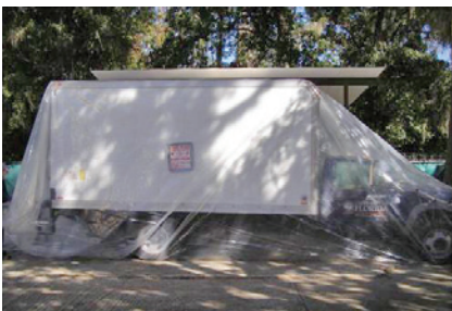
FIGURE 12 • Fumigation chamber wrapped in polyethylene sheeting.
