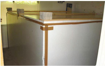
FIGURE 10 • A “heat chamber” made of insulated polystyrene sheets built around a pile of furnishings.
